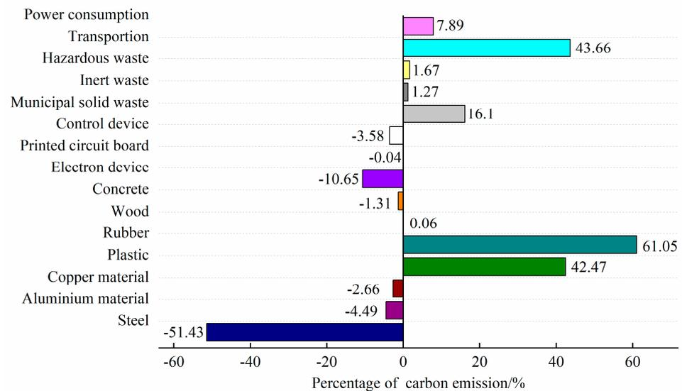
**Figure 6.** Percentage of the carbon dioxide emissions during the demolition and scrapping stage.
