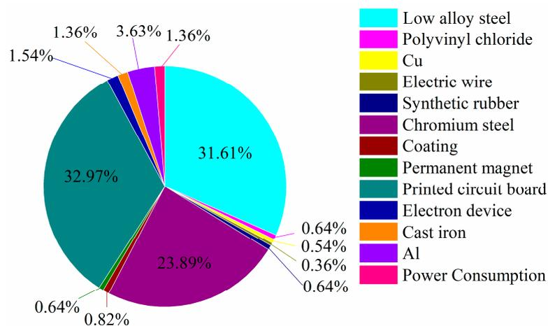
Figure 3. The percentages of carbon dioxide emissions in the manufacturing stage.
