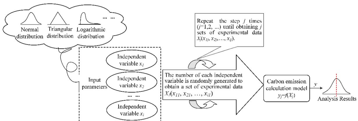
Figure 2. Monte Carlo simulation method.
