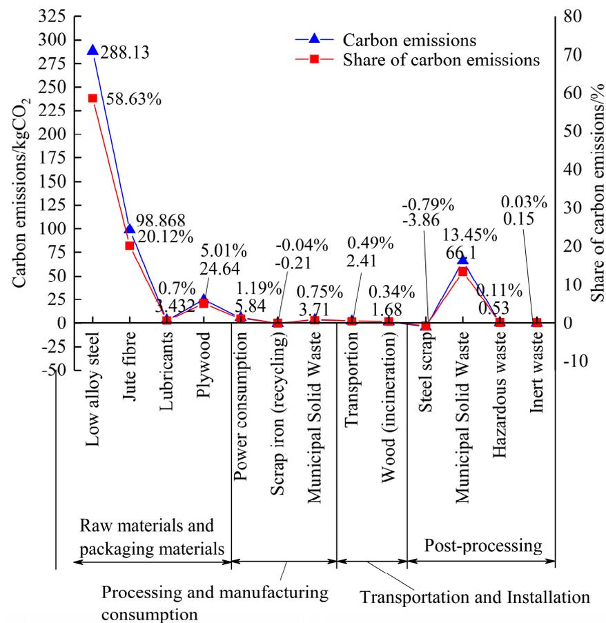
**Figure 5.** Carbon dioxide emissions and shares during the maintenance stage.
