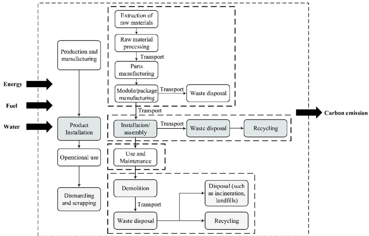
**Figure 1.** Carbon dioxide emissions framework of the elevator in different stages.
