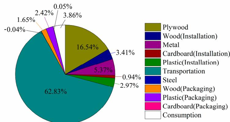
Figure 4. The percentage of the carbon dioxide emissions at the product installation stage.
