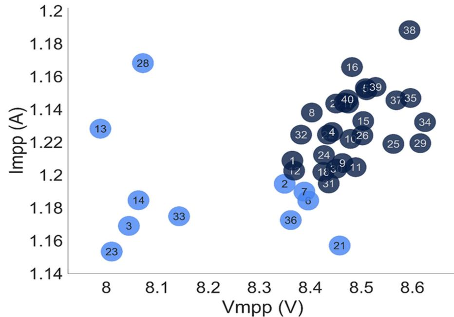
**Figure 7.** The relationship between  $V_{mpp}$  and  $I_{mpp}$  of non-uniformly-aged forty polycrystalline PV modules dataset. The module number with light blue colors represents the mostly aged module and dark blue color modules are slowly degraded.
