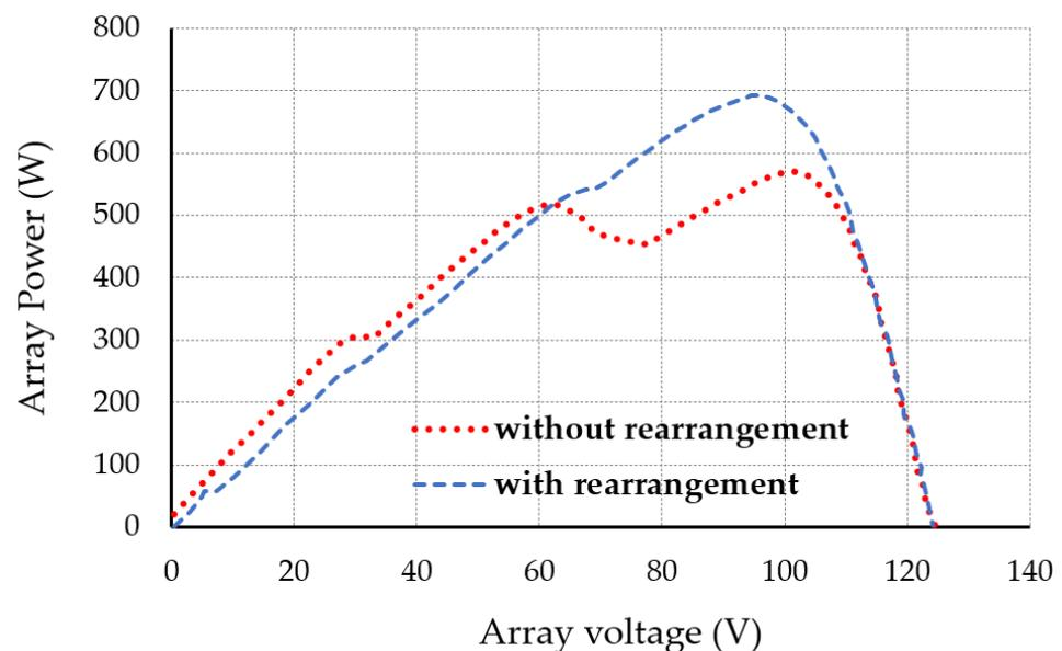
Figure 1. Power increment of PV array modules under non-uniform aging conditions [39].
