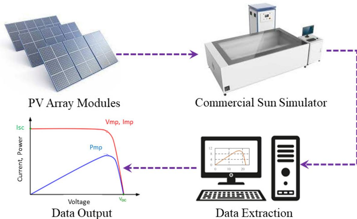
**Figure 6.** Aged PV module testing system in the solar module manufacturer company.
