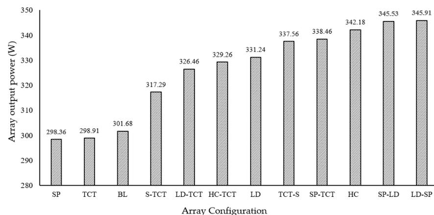
**Figure 12.** Comparison of power outputs among different array configurations for  $4 \times 10$  array.
