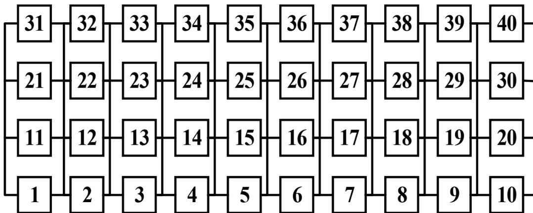
**Figure 10.** TCT configuration is used to connect  $4 \times 10$  array modules. The SCC approach chooses and arranges the PV modules' positions.
