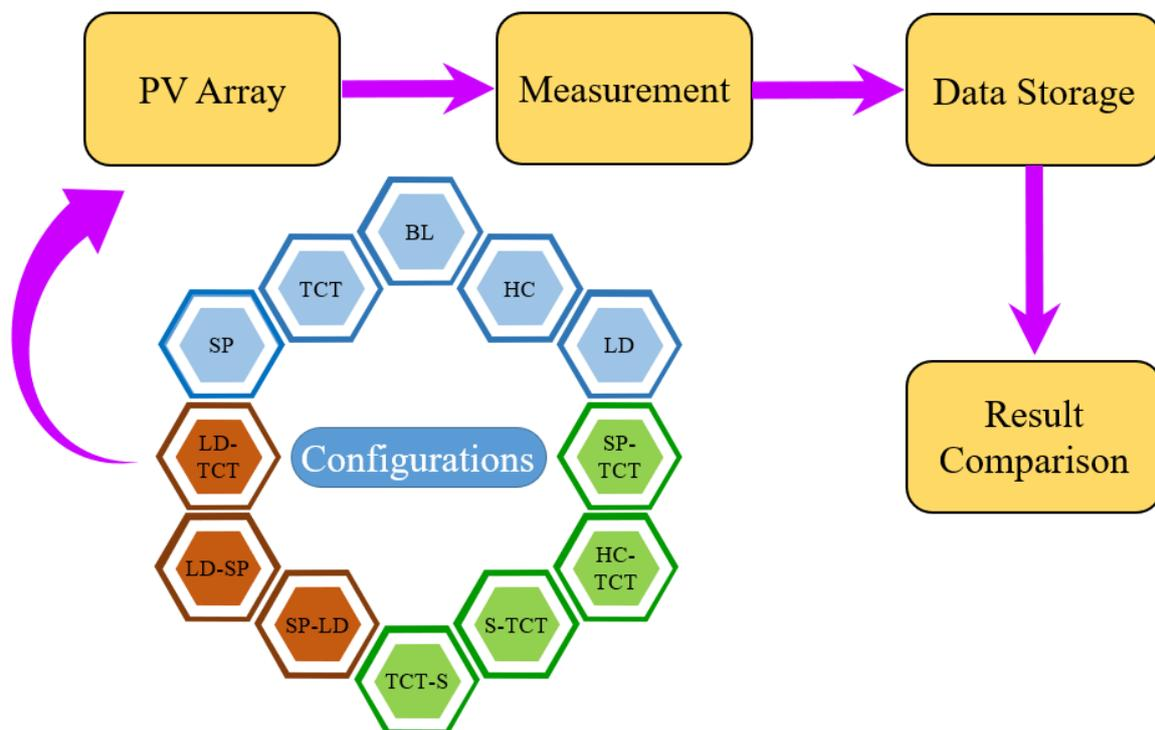
**Figure 2.** The conventional and proposed configurations are tested using an aged PV array. The array modules are rearranged via the SCC method. The output characteristics of the PV array are measured using PROVA 1011 for each configuration to make the result comparison.
