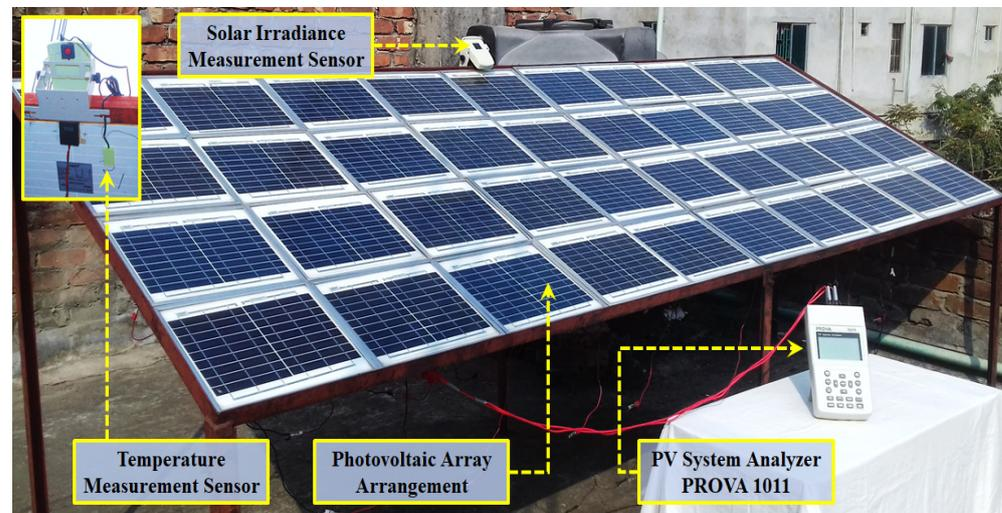
**Figure 11.** Experimental data collection of the non-uniformly-aged PV array. Each configuration is applied to make the module interconnection, and output electrical characteristics are measured using the PROVA 1011.
