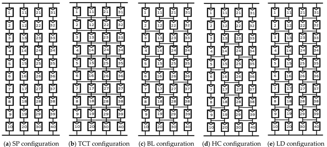
Figure 3. Standard configurations of  $4 \times 10$  PV Array.
