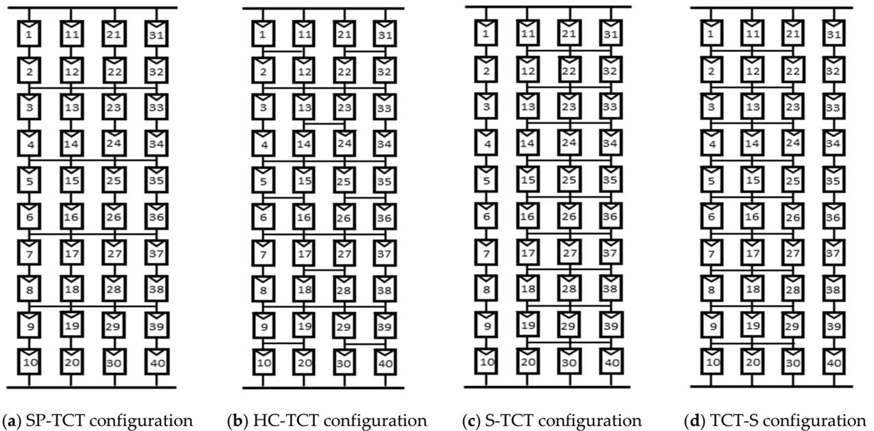
Figure 4. Hybrid Configurations of  $4 \times 10$  Array.
