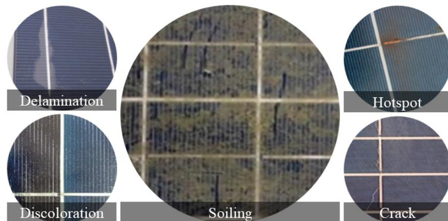
**Figure 9.** The five common non-uniform aging factors delamination, discoloration soiling, hotspot, and cell crack are shown here from the 4 years of the aged 40 PV modules. Most of the PV modules are degraded by these types of aging factors.
