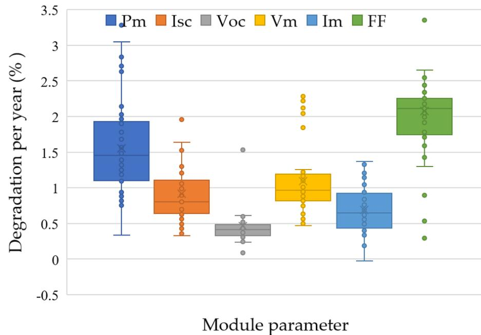
**Figure 8.** The degradation rate of different electrical parameters of aged photovoltaic modules.
