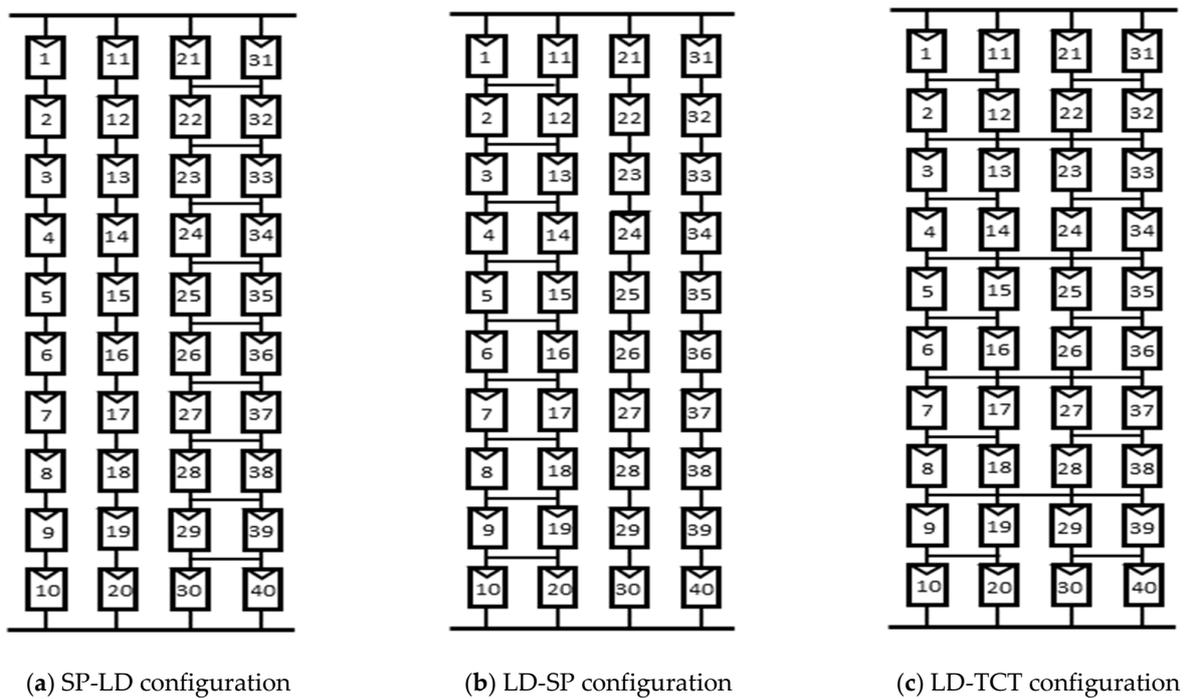
Figure 5. Proposed Hybrid Configurations of  $4 \times 10$  Array.
