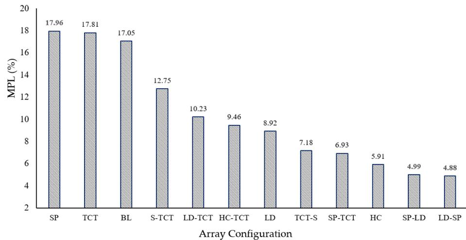
**Figure 13.** Comparison of MPL% among different array configurations for  $4 \times 10$  array.
