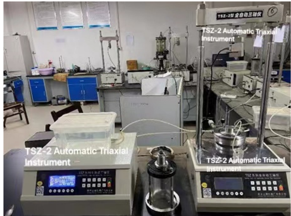
Figure 2. TSZ-2 fully automatic triaxial instrument.
