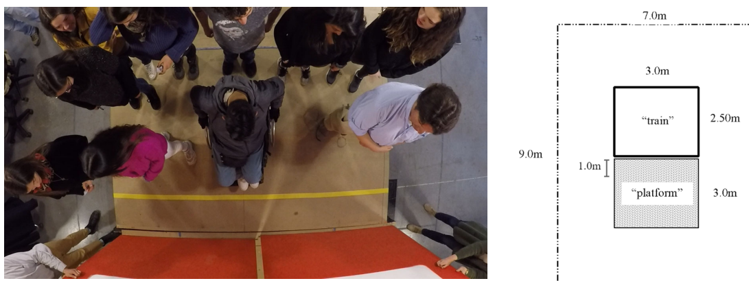
Figure 4. Mock-up in the controlled environment: platform (left); PTI layout (right).
