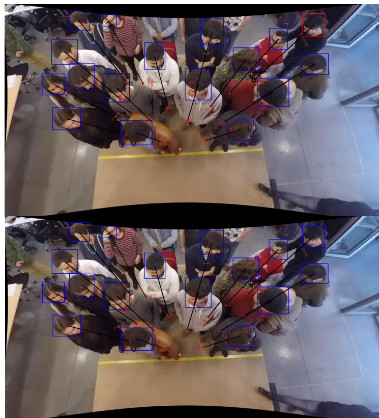
Figure 6. Images of passengers waiting to board, considering the same situation of H = 2.7 and \varphi = 14^\circ but under different values of h . For the upper image, h = 1.65 m (16 detections shown by blue squares within the area of interest and 1 detection shown by the red square out of the area of interest), while in the lower image, h = 1.75 m (17 detections shown in blue squares within the area of interest).
