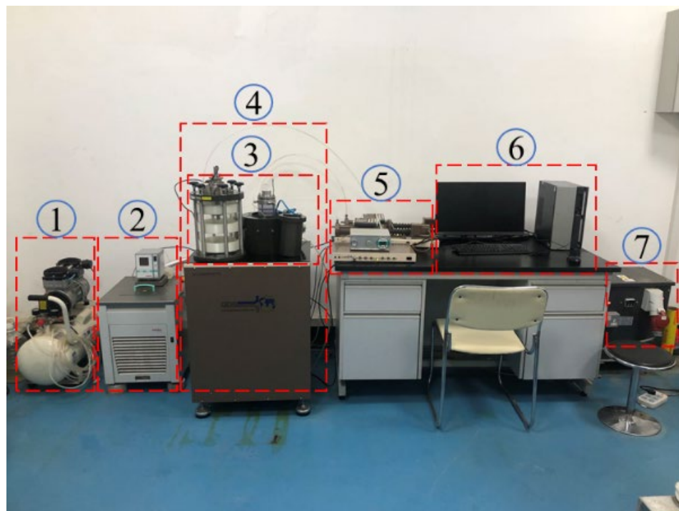
Figure 1. Triaxial test system with temperature-controlled vibration. ① is a pneumatic pump; ② is a temperature control system; ③ is a pressure chamber with temperature monitoring; ④ is a dynamic triaxial testing machine; ⑤ is a data acquisition system; ⑥ is a computer monitor; ⑦ is the transformer of the dynamic triaxial testing machine.
