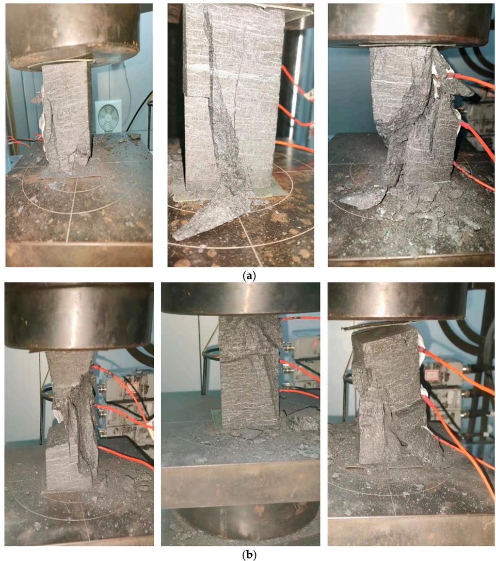
**Figure 4.** Mode of failure: (a) Natural samples; (b) Water-saturated samples.
