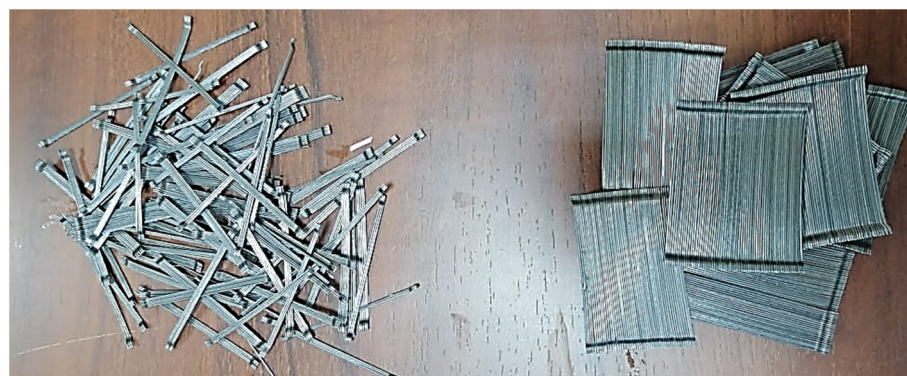
Figure 3. Bundled steel fibers.
