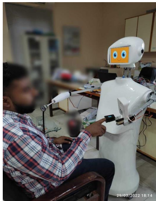
Figure 26. Demonstration of RoboDoc taking the pulse rate and SpO2 level of a subject and RoboDoc taking data (similar to Figure 25b).
