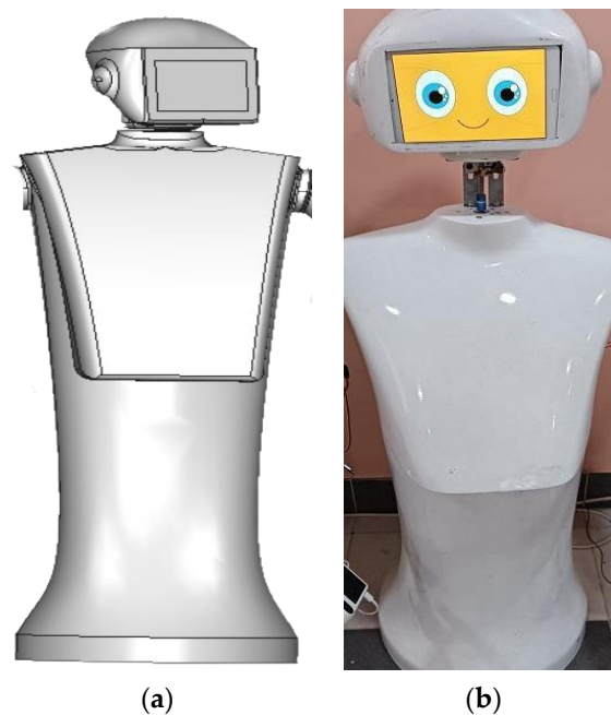
Figure 7. Torso: (a) CAD Design; (b) Physical Design.
