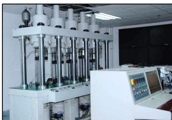
Figure 2. The Five-link Rheological Test System for Deep Soft Rock.
