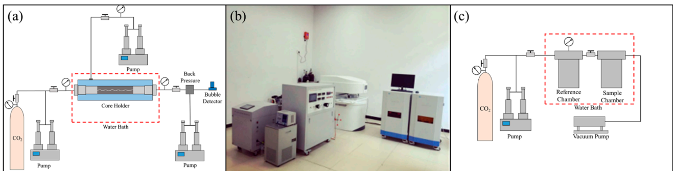
Figure 3. The experiment apparatus. (a) The BP experiment system. (b) NMR experiment system. (c) The isothermal adsorption experiment system.
