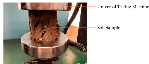
Figure 4. Unconfined compression test.
