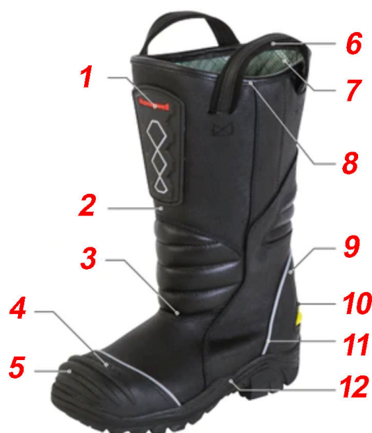
Figure 16. Firefighter's footwear NightHawk™ 5555 PRO Series from Honeywell. Explanatory notes: 1. Rubber Shin Guard, 2. Heavyweight Kevlar, 3. Premium Full-Grain Cowhide Leather, 4. Power Toe Protection, 5. Oblique Steel Toe Cap, 6. Leather-Reinforced Pull Straps, 7. Footwear Fabric Lining, 8. Leather Top Binding, 9. Heel and Ankle Grip System, 10. Heel Kicker, 11. Reflective Trim, 12. Rugged Reliable Protection.
