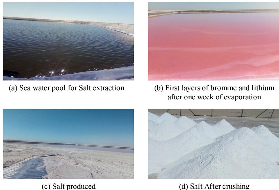
Figure 6. Salt production at Duqm Salts Factory, Oman.
