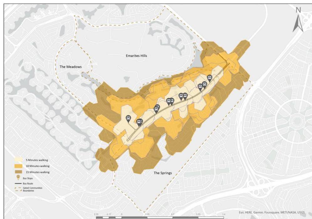
Figure 18. The bus stops walkability within 5, 10, and 15 min for the Springs and the Meadows.
