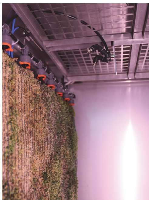
Figure 5. Drip irrigation at the upper end of the panel.
