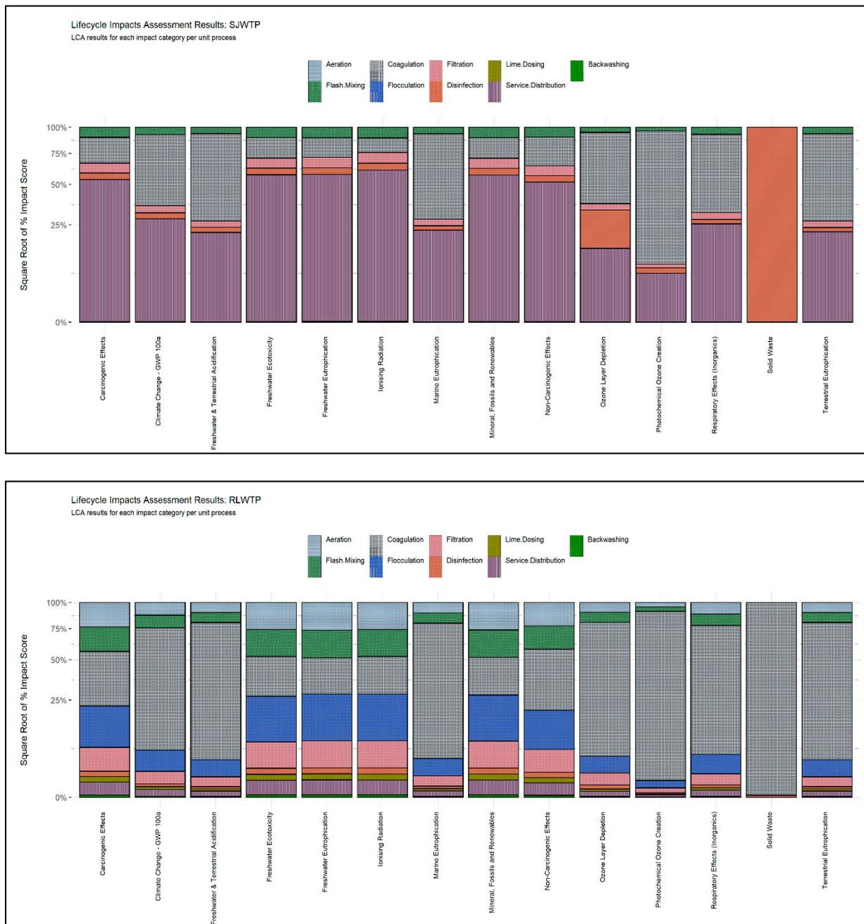
**Figure 3.** Life cycle impact results for SJWTP (top) and RLWTP (bottom). Distinct unit treatment processes are represented by color schemes with respect to the life cycle impact categories.
