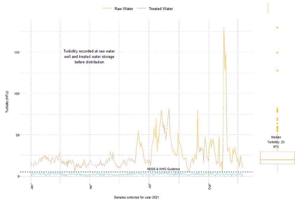
**Figure 2.** Water quality at the RLWTP for the year 2021. Left: Line plot of raw and treated water turbidity variation over 12-month period. Right: Box plot for the raw water turbidity.
