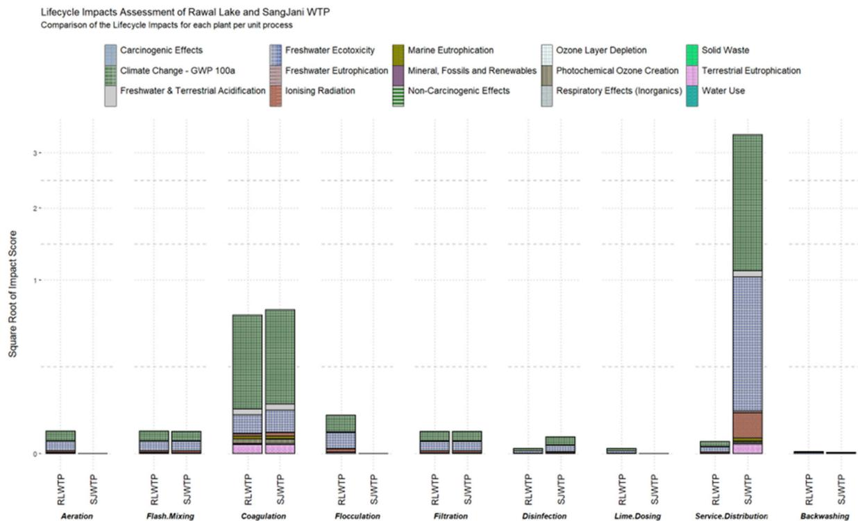
**Figure 8.** Comparative analysis of the life cycle impacts calculated for both the water treatment plants. The impacts are presented with respect to each impact category, with a relative comparison of both systems.
