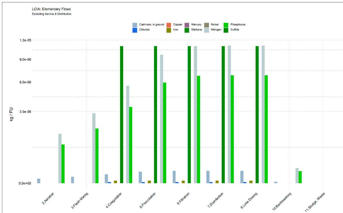
**Figure 4.** Cumulative life cycle impact results for each treatment process. Selected elementary flows are represented with distinct colors. The emission compartments mainly include air and water. The scale represents the emission concentration per functional unit.
