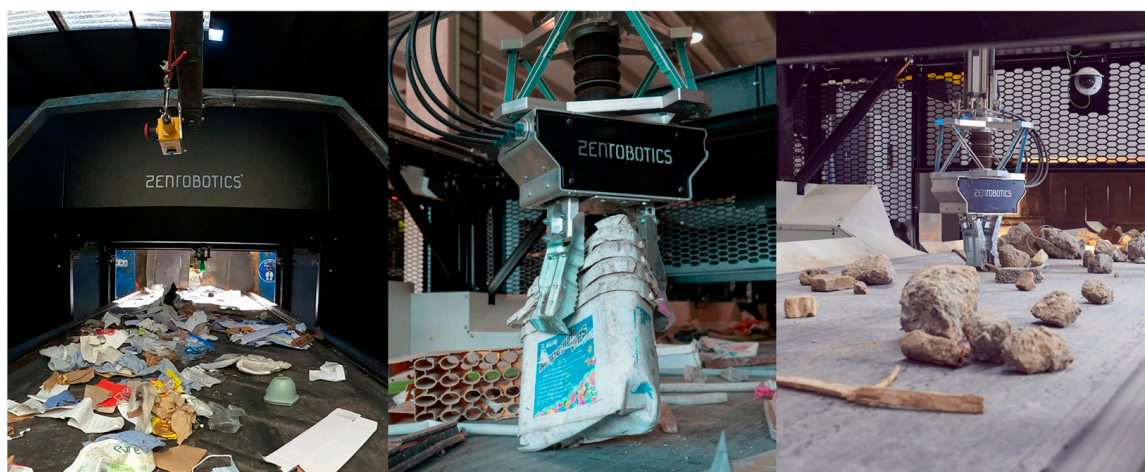
Figure 2. ZRR2 robot applied in garbage sorting [35].
