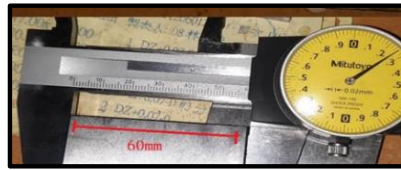
Figure 3. Schematic of Dimensional Error Due to Misreading Order (Order dimension is 58 mm, but actual measurement is 60 mm).
