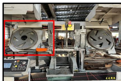
Figure 14. Schematic of Saw Blade Wheel (Box highlights the saw blade wheel).
