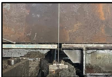
Figure 12. Schematic of Uneven Bed.
