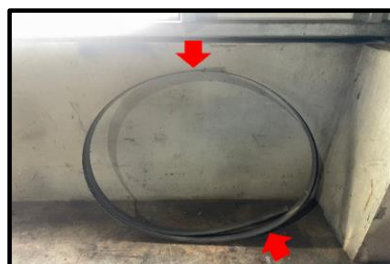
Figure 7. Schematic of Saw Blade Breakage (Arrow indicates the breakage area).
