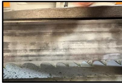
Figure 8. Schematic of Saw Blade Tooth Damage.
