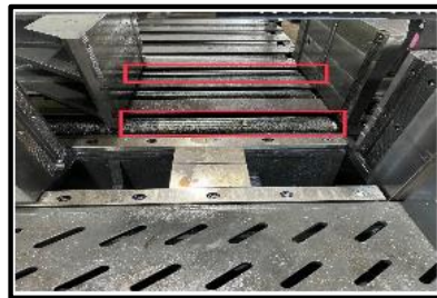
Figure 5. Schematic of Linear Slide Rail/Screw Rail Failure (Box highlights the slide rail).
