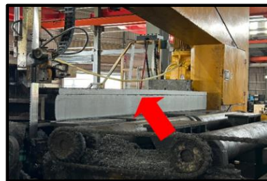
Figure 1. Steel Plate Surface Deformation (Arrows indicating the deformation area).
