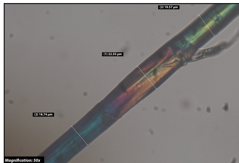
Figure 4. Amorphous and crystalline regions of N-HEMP fibre under the microscope.
