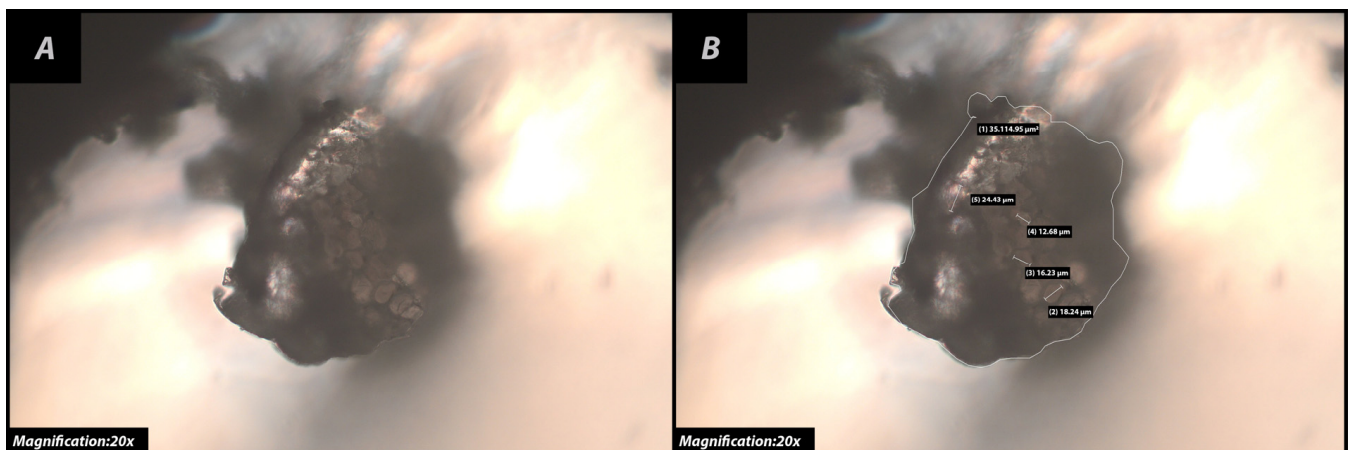
Figure 6. (A) N-HEMP cross-sectional view without the fibre diameters. (B) N-HEMP cross-sectional view with the fibre diameters.
