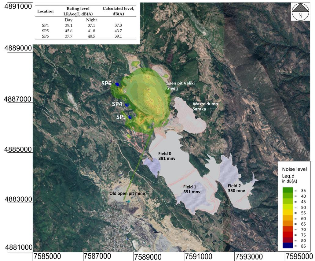
Figure 3. Noise levels estimation around the open-pit mine Veliki Krivelj for the model validation.
