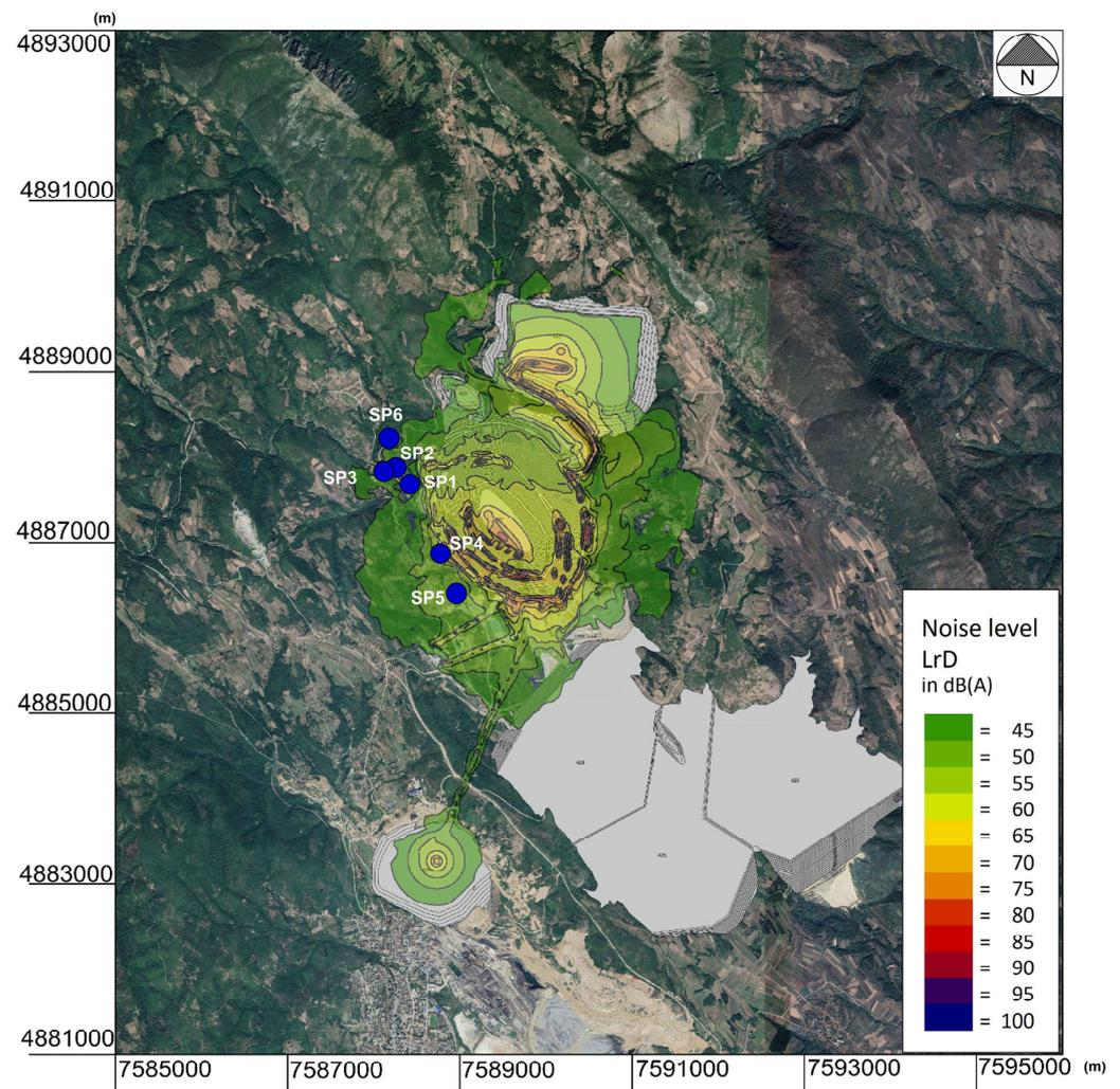
**Figure 5.** The night noise level estimation on sensitive points SP1–SP6 and around the open-pit mine Veliki Krivelj, resulting from modeling different spatial organization of work in the mine.
