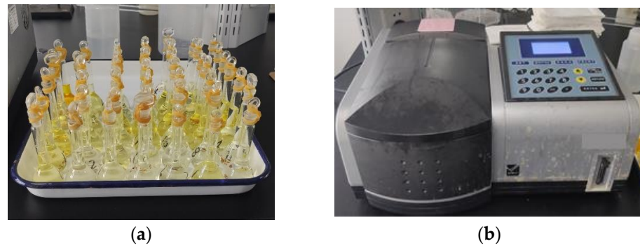
Figure 7. PGENERAL UV-Vis spectrophotometer and samples to be tested: (a) UV-V is the spectrophotometer; and (b) Colorimetric test sample.
