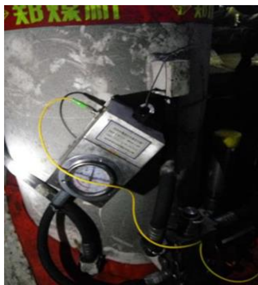
Figure 13. Field installation diagram of FBG manometers.
