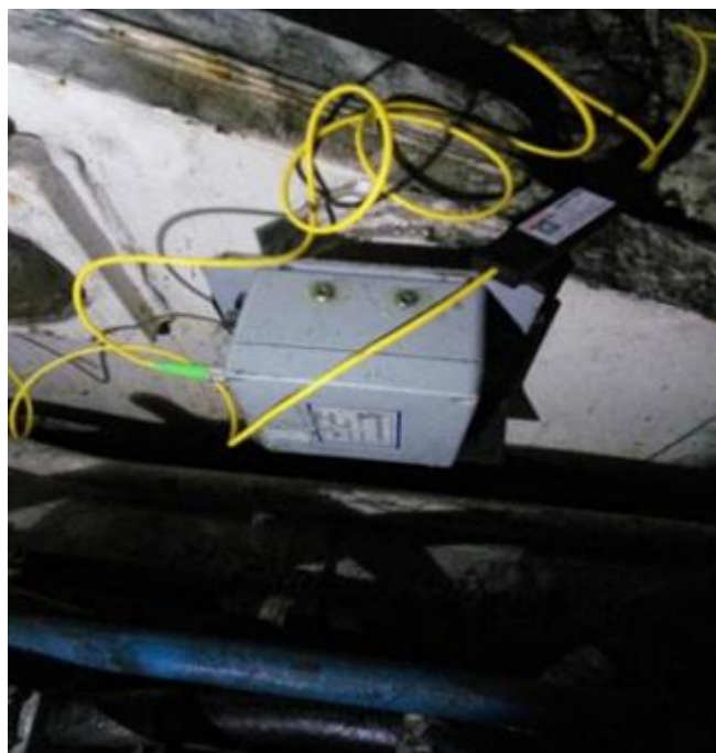
Figure 12. Field installation diagram of FBG tilt sensors.
