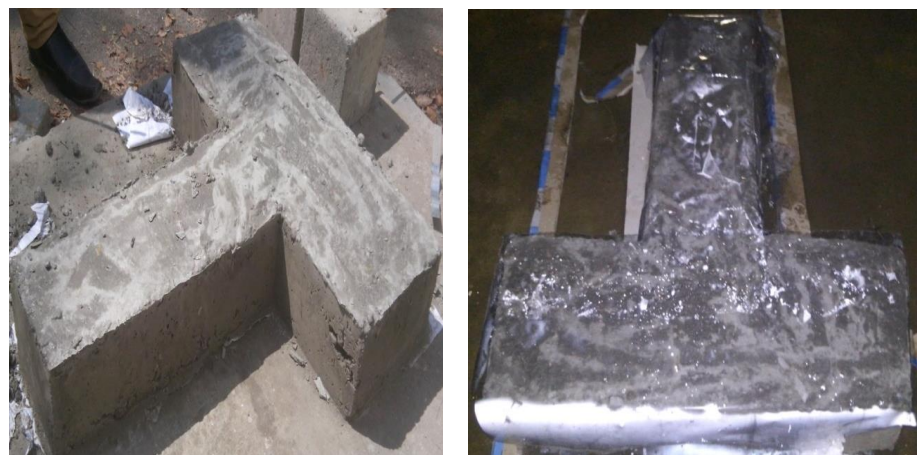
Figure 2. Curing of the Beam Column joint specimen.
