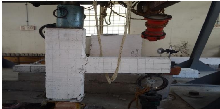
(b) Reverse loading setup of the beam column joint.
