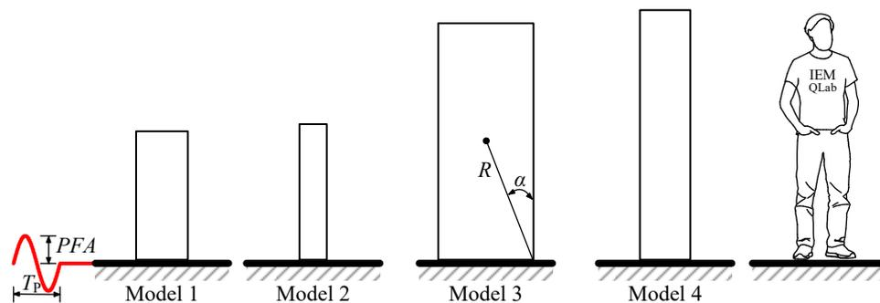
Figure 7. Schematic illustration of the investigated rocking block geometries.
