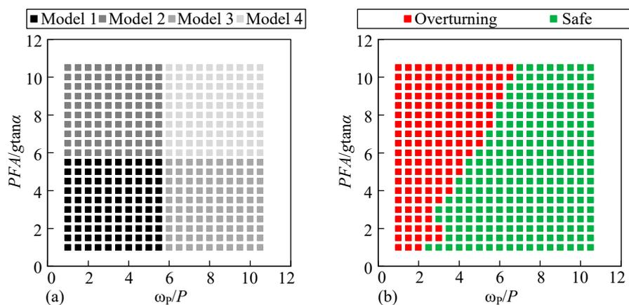
Figure 8. (a) Model distribution and (b) seismic responses of blocks subjected to one-sine pulse.
