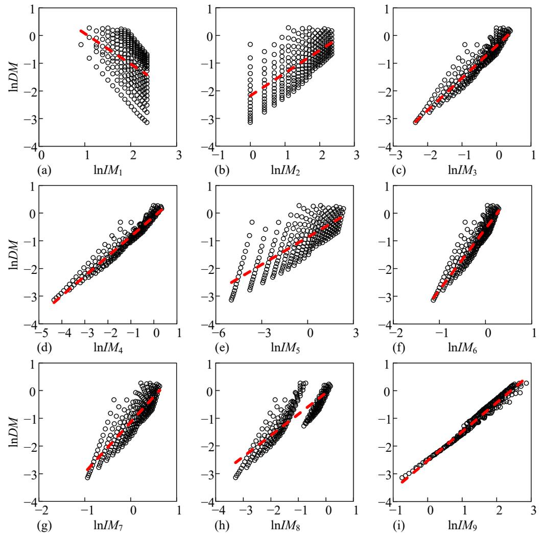
Figure 11. Linear regression analysis of the maximum normalized response with respect to different IMs: (a–h)  $IM_1$ – $IM_8$ ; (i) the proposed  $IM_9$ .
