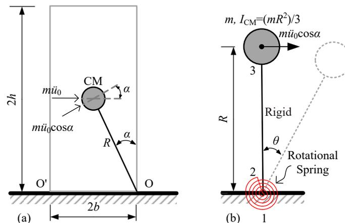
**Figure 3.** (a) Lumped mass representation of rigid block and (b) equivalent SDOF model of a rigid rocking block.
