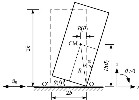
Figure 1. The geometry of a rocking block.
