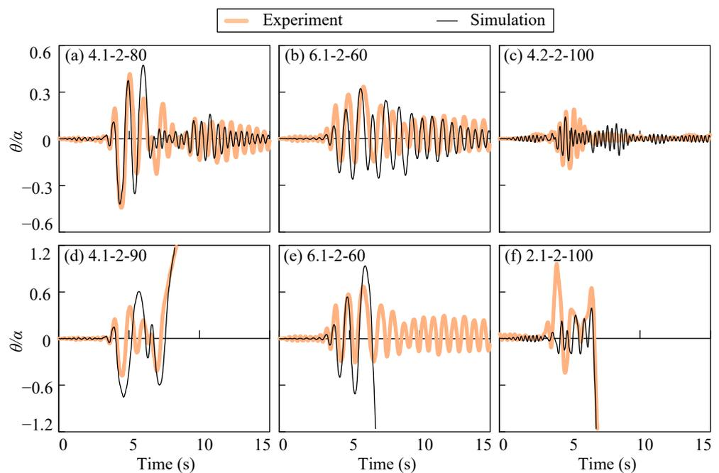
**Figure 6.** Comparison of rotation histories of non-overturning (a–c) and overturned (d–f) runs by SDOF models.
