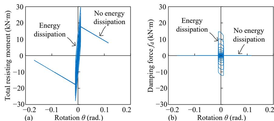
**Figure 4.** Hysteretic curves of a free-rocking SDOF system of  $\alpha = 0.2$  and  $R = 0.38$  m: (a) total resisting moment with discrete damping, (b) discrete damping force.
