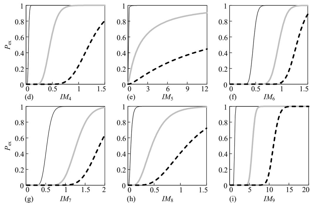
**Figure 12.** Rocking fragility curves for different IMs: (a–h)  $IM_1$ – $IM_8$ ; (i) the proposed  $IM_9$ .
