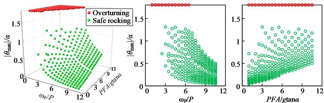
Figure 9. Three-dimensional rocking rotation spectrum.
