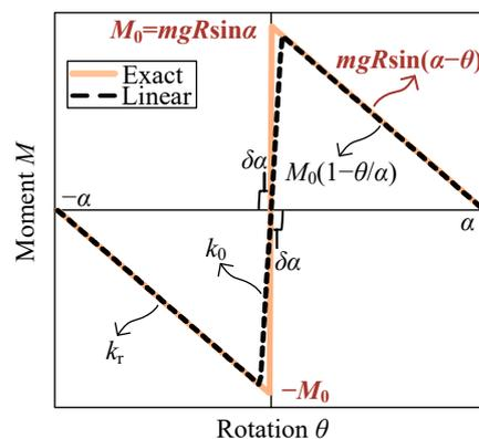
Figure 2. Moment-rotation relationship of a rocking block.
