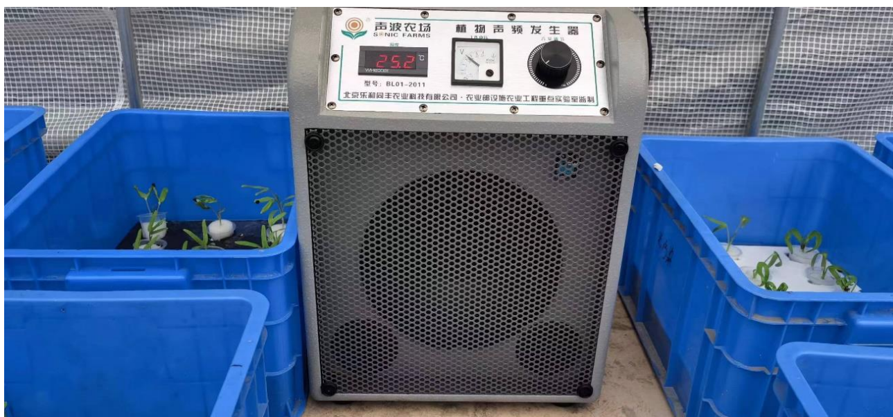
Figure 6. The fully automatic first-generation Plant acoustic frequency technology generator (AFT model: BL01-2011).
