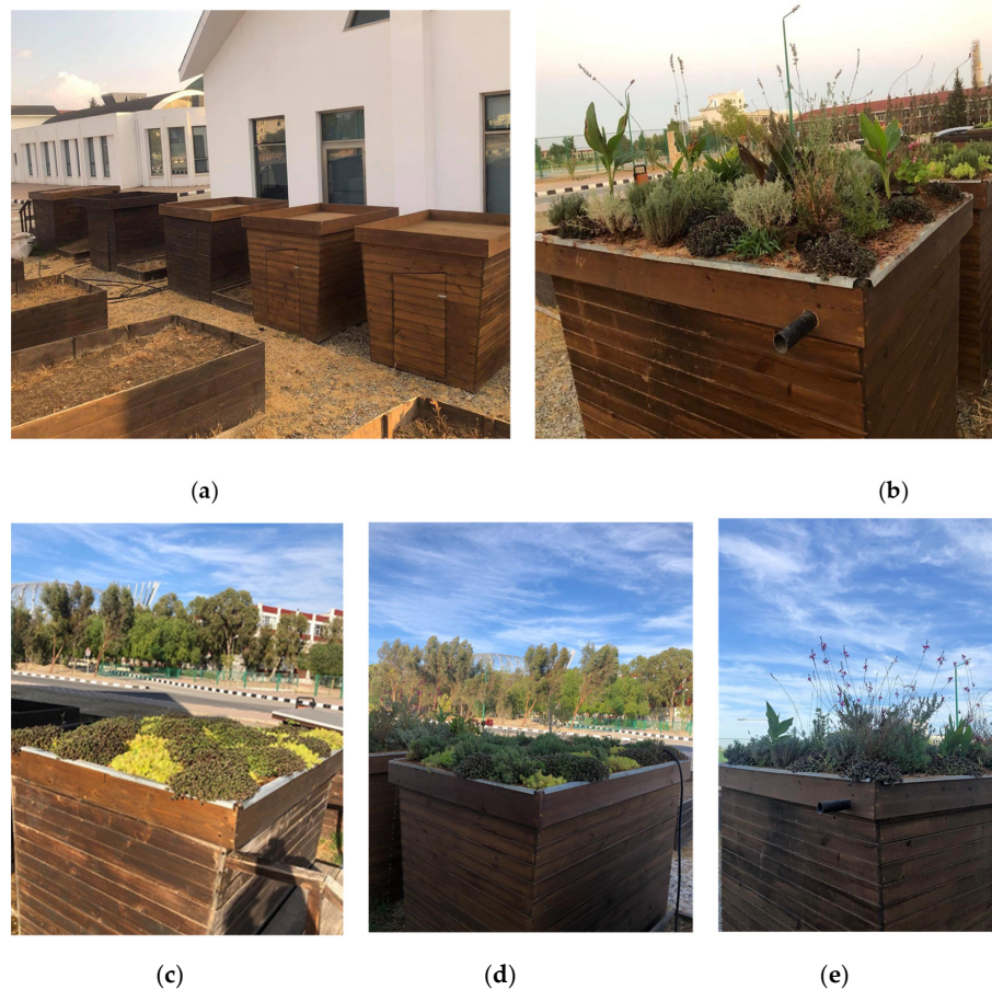
Figure 2. (a) The huts used in the green roof; (b) all green roof huts, including the control hut used in the comparison; (c) green roof with ground-covers; (d) green roof with mixed vegetation; (e) green roof with shrubs.
