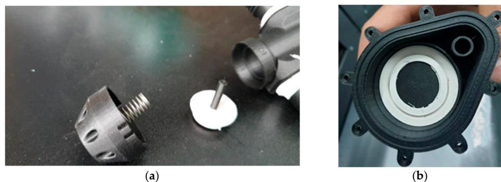
**Figure 11.** (a) A produced series of springs; (b) casted silicone diaphragms.
