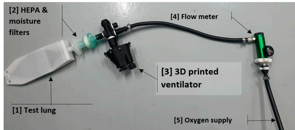
**Figure 12.** Final assembly including: 1. a test lung; 2. HEPA and moisture filters; 3. the ventilator; 4. a flow meter; 5. the oxygen supply.
