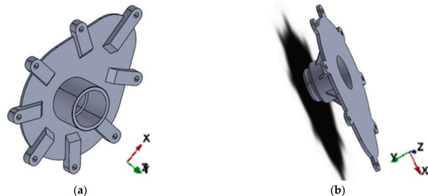
**Figure 5.** (a) Initial CAD of the top modulator; (b) final CAD of the top modulator.
