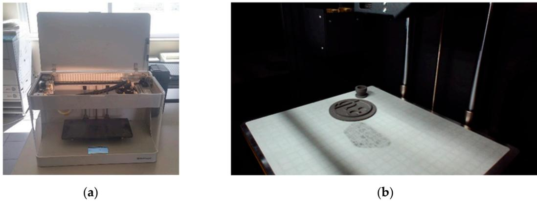
**Figure 9.** (a) MarkForged Composite Nylon printer; (b) Metal-X printer.
