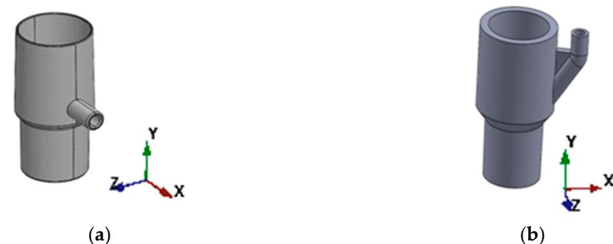
**Figure 6.** (a) Initial CAD of the manometer body; (b) final CAD of the manometer body.
