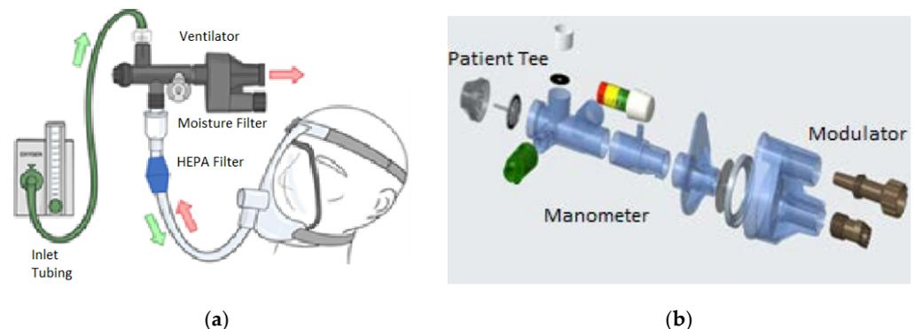
**Figure 1.** (a) Schematic of the oxygen flow; (b) exploded view of the ventilator assembly (modified from [15,16]).
