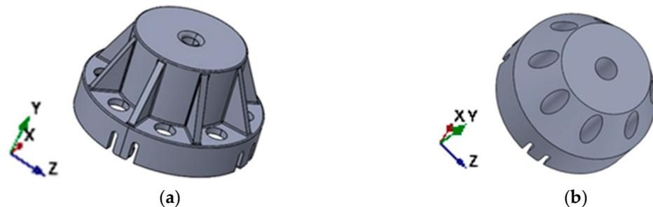
**Figure 8.** (a) Initial CAD of the pop-off valve cap; (b) final CAD of the pop-off valve cap.
