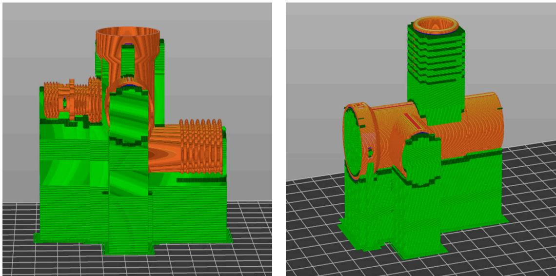
Figure 2. The supports needed (in green color) in two possible printing orientations.
