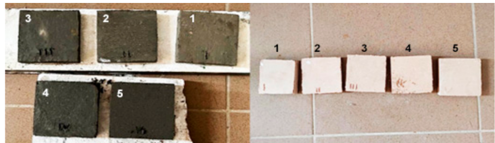
Figure 2. Glass ceramic samples before and after the heat treatment at 900 °C.
