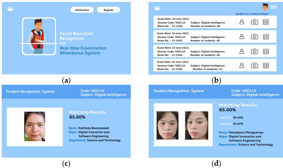
Figure 2. Samples of biometric recognition interfaces for examination attendance system: (a) the home page of the system; (b) examination information sessions; (c) the screen of a unimodal recognition result; (d) the screen of a multimodal recognition results.
