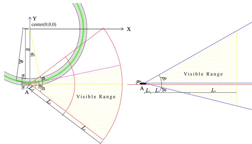
**Figure 2.** Schematic representation of the visual field volume of the roadside landscape on a curved highway.
