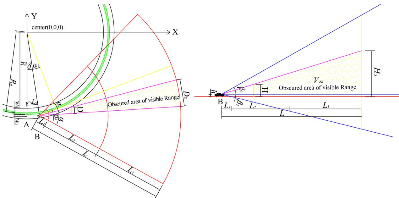
**Figure 4.** Schematic representation of the occluded volume of the visual field of the roadside landscape on a curved highway (volume at time  $t_i$ ).
