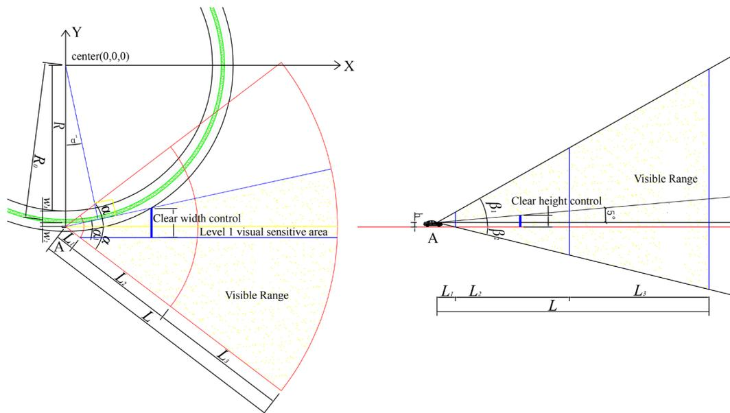
**Figure 10.** Schematic diagram of roadside landscape clearance control for a curved highway.
