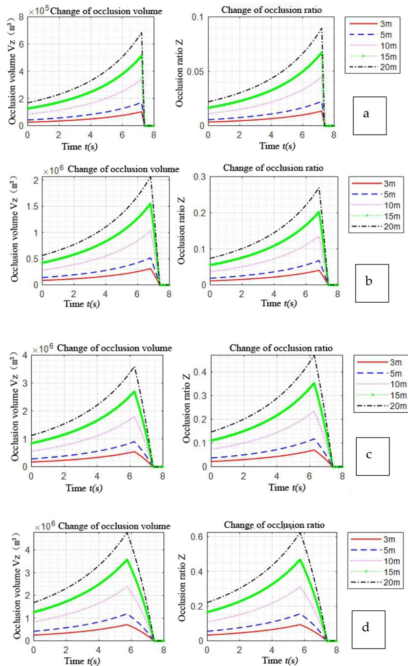
**Figure 8.** Simulation of the change of the occlusion volume and occlusion ratio of the roadside landscape by the occlusions of different heights under the same main line design speed, the same position, and the same width: (a) Obstruction of different heights when  $D = 3$  m; (b) Obstructions of different heights when  $D = 10$  m; (c) Obstructions of different heights when  $D = 20$  m; (d) Obstructions of different heights when  $D = 30$  m.
