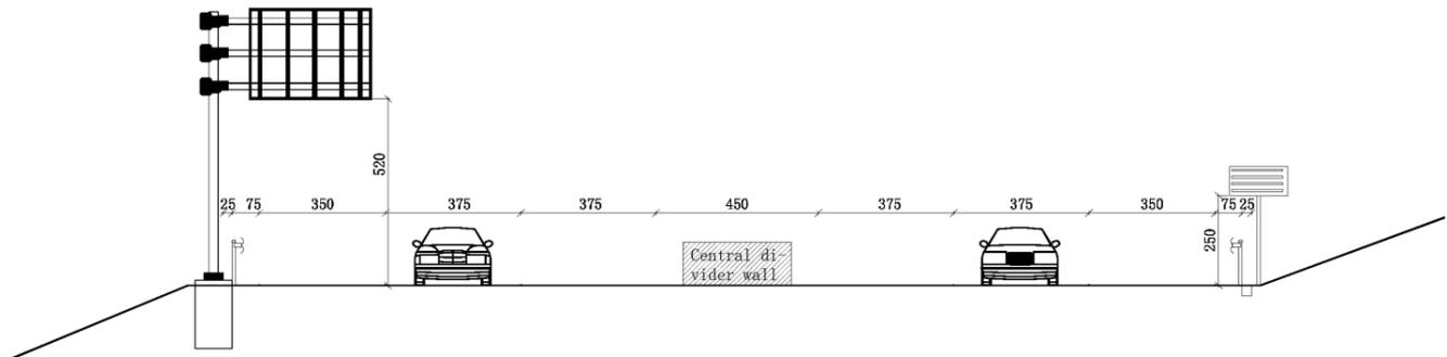
Figure 7. Typical standard cross section of G4 Hunan section (unit: cm).
