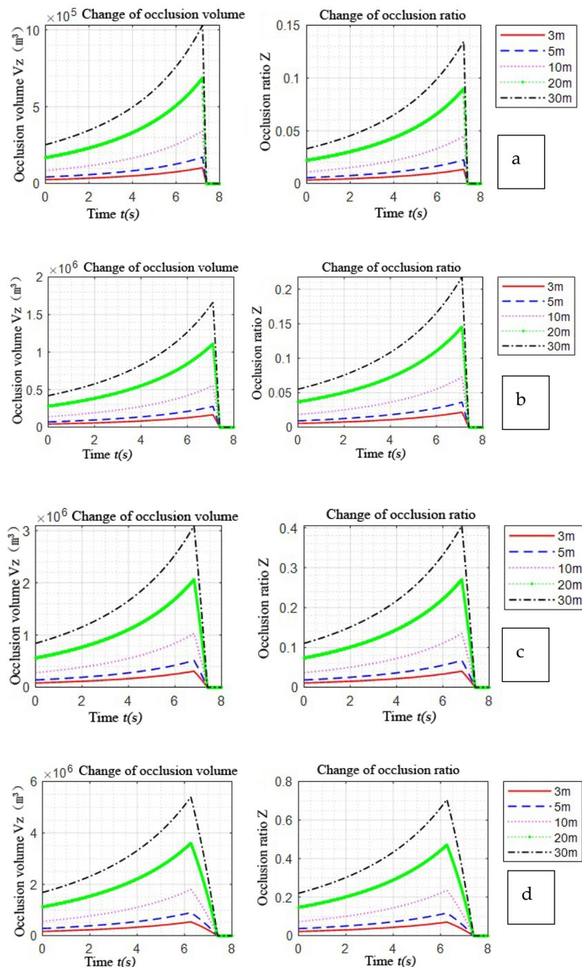
**Figure 9.** Simulation of the change of the occlusion volume and occlusion ratio of roadside landscape by occlusions of different widths under the conditions of the same main line design speed, the same position, and the same height. (a)  $H = 3$  m with different widths of obstruction; (b)  $H = 5$  m with different widths of obstruction; (c)  $H = 10$  m with different widths of obstruction; (d)  $H = 20$  m with different widths of obstruction.
