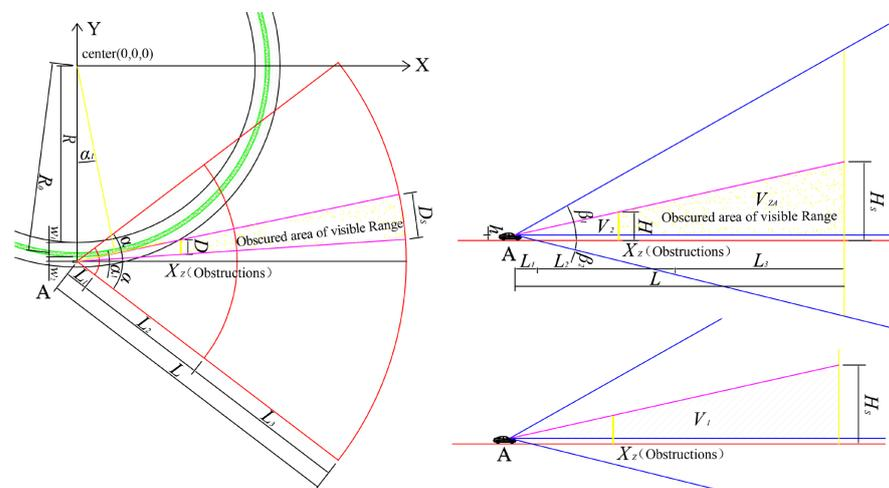
**Figure 3.** Schematic representation of the occluded volume in the visual field of the roadside landscape (point A).
