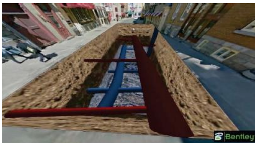
Figure 2. AR application in earthwork stage [18].
