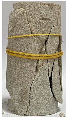
Figure 7. Failure image of cylinder white sandstone specimen under quasi-static loading (The loading direction is vertical).
