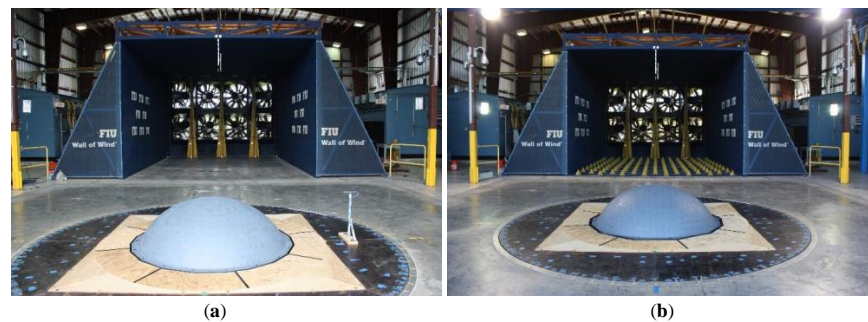
Figure 6. (a) Open terrain configuration with spires; (b) Suburban terrain configuration with both spires and surface roughness elements.
