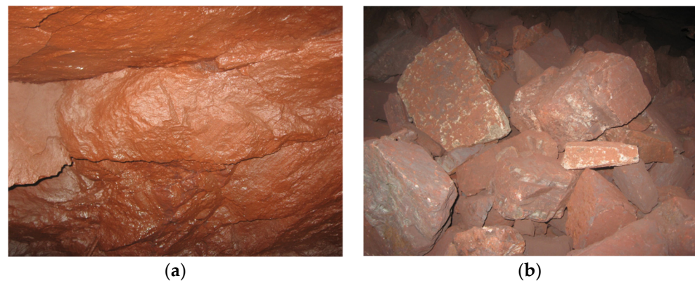
Figure 3. Photographs of cracks in the ore mass (a) and pieces of the backfilling material in the pipe (b).
