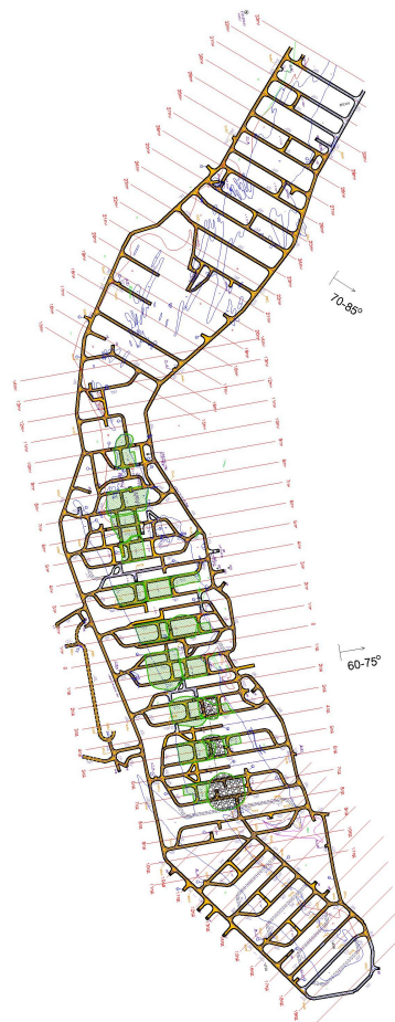
Figure 1. Section of the ore deposit with mining operations along the extracting horizon, 875 m.
