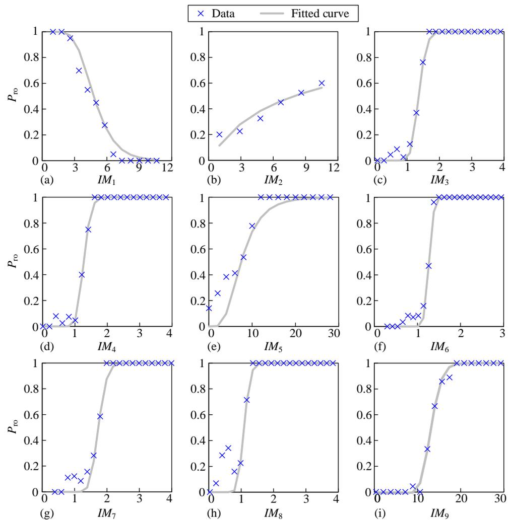
Figure 10. Overturning fragility curves for different IMs.
