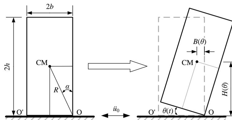
Figure 1. Rocking block geometry.
