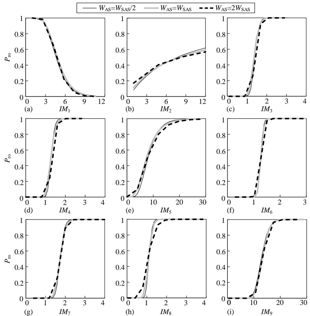
Figure 12. Overturning fragility curves for different widths of the analysis strips.
