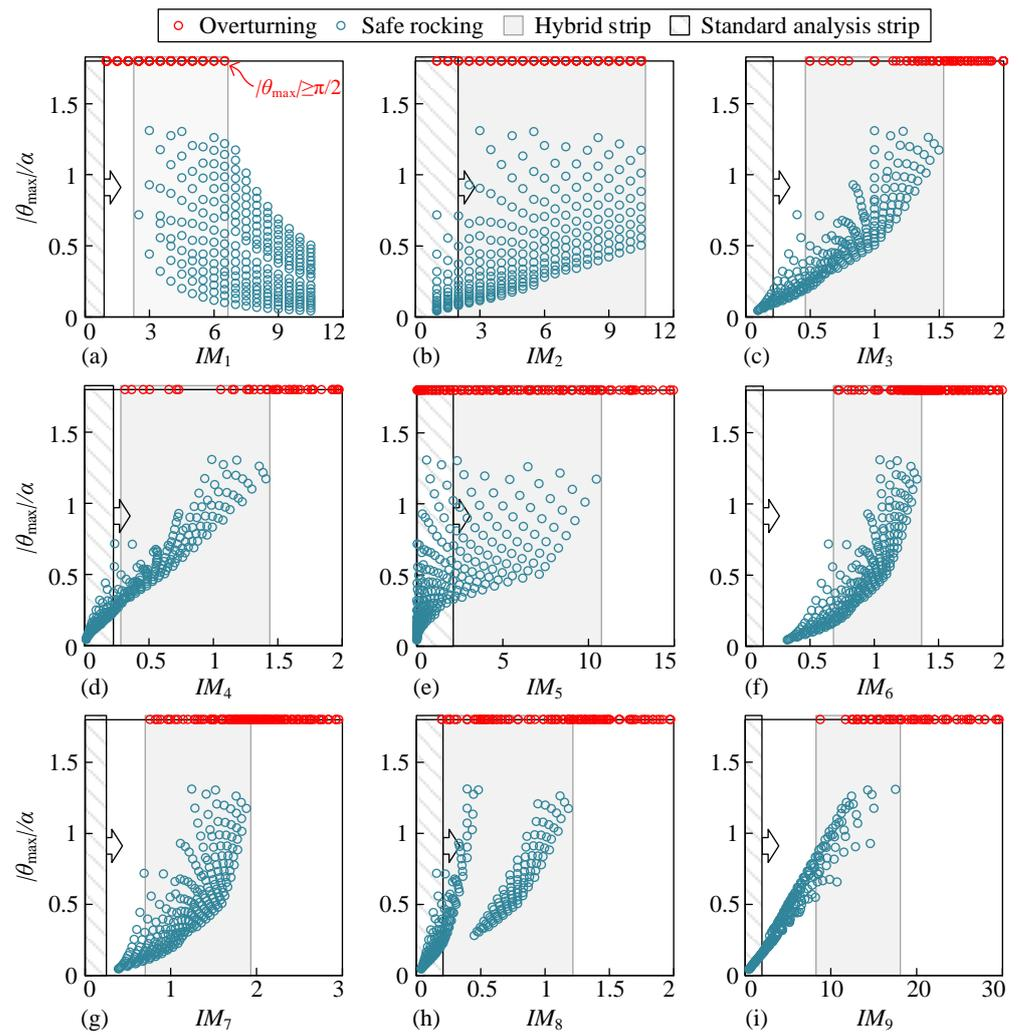
Figure 8. Seismic response analyses for different IMs.
