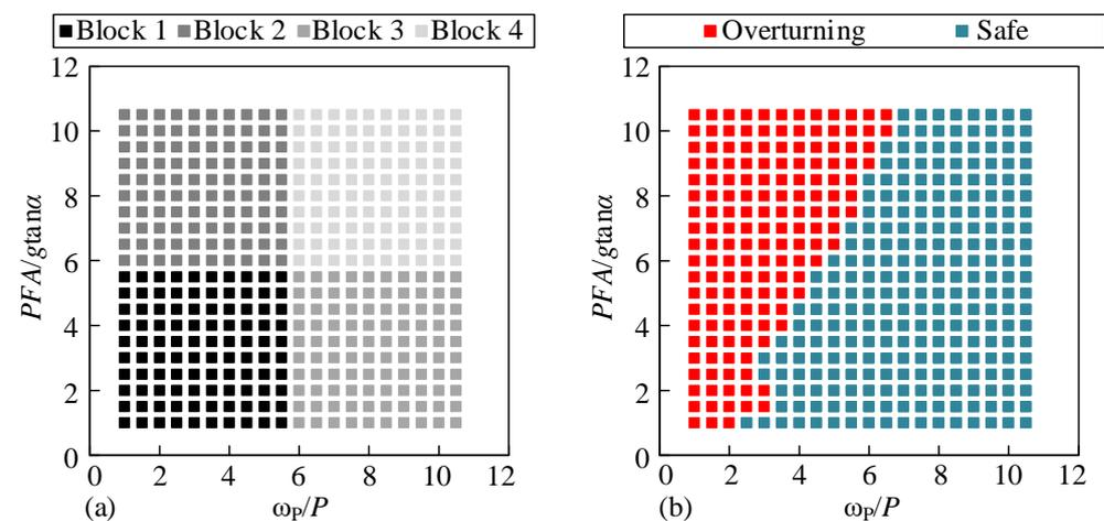
Figure 6. (a) Model distribution and (b) overturning spectrum.
