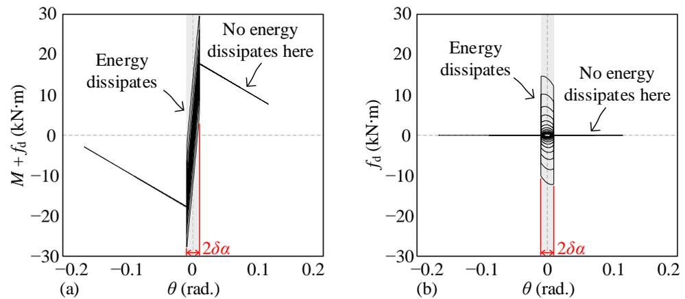
**Figure 3.** Hysteresis of the SDOF model: (a) total resisting moment vs. rocking angle, (b) damping force vs. rocking angle.
