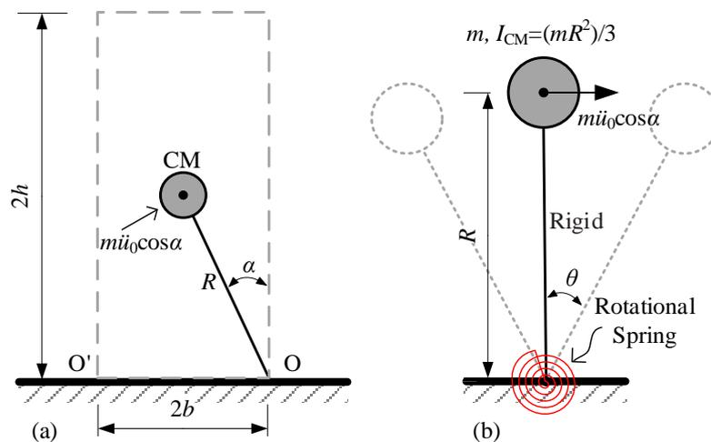
Figure 2. (a) Rigid block and (b) equivalent SDOF model.
