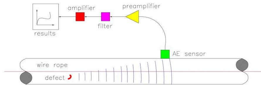
**Figure 6.** Principles of typical AE testing method for wire rope.
