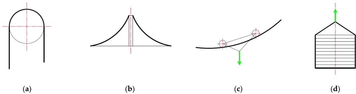
**Figure 2.** Types of ropes according to their use: (a) running rope; (b) stationary rope; (c) track rope; (d) rope sling.
