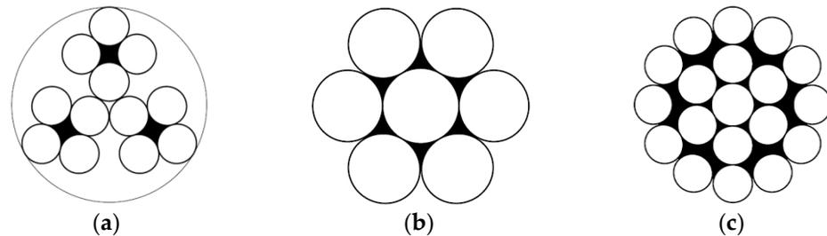
**Figure 1.** Basic structures of steel wire ropes/strands: (a) structure of Albert's rope; (b) strand 1 + 6; (c) strand 1 + 6 + 12.
