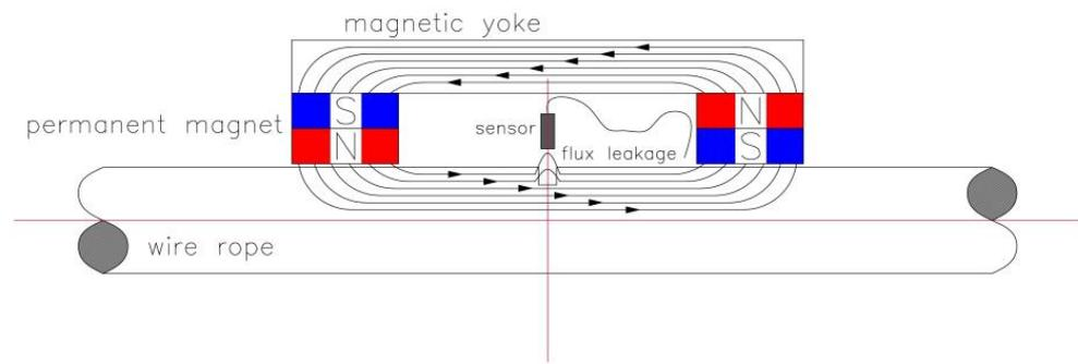
**Figure 4.** Principles of typical MFL testing method for wire rope.
