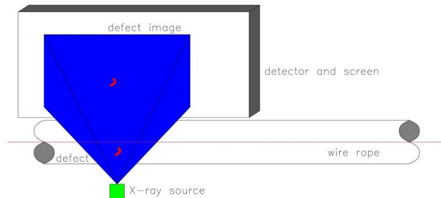
**Figure 8.** Principles of typical radiography testing (X-ray source) method for wire rope.
