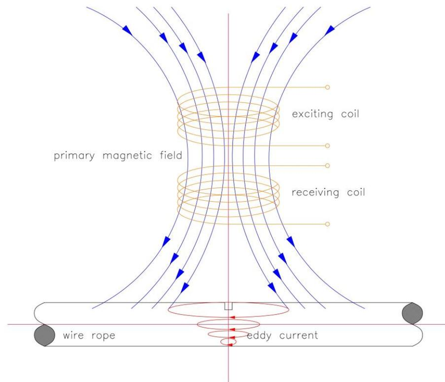
**Figure 5.** Principles of typical ECT method for wire rope.
