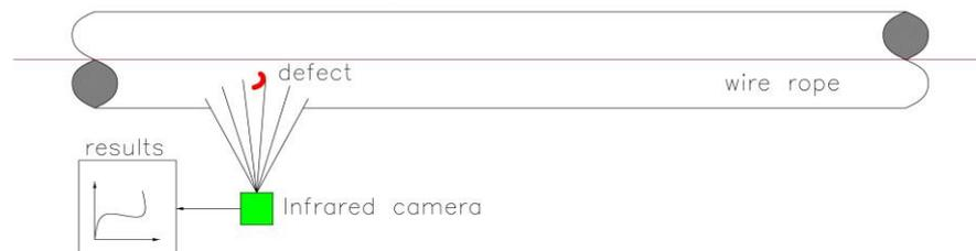
**Figure 9.** Principles of typical induction thermography method for wire rope.
