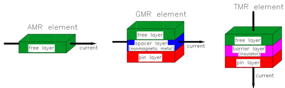
**Figure 10.** Different structures of MR sensors.
