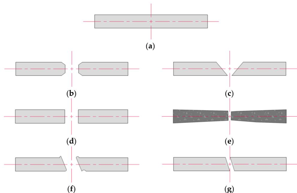
**Figure 3.** Types of LF loss: (a) no loss; (b) overload; (c) wear; (d) fatigue; (e) rust; (f) kink; (g) cut.
