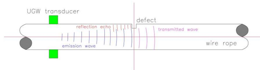
**Figure 7.** Principles of typical UGW testing method for wire rope.
