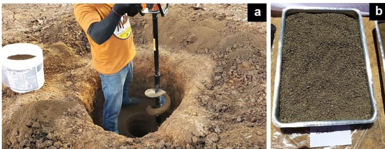
Figure 1. Clay collection process (a), followed by a portion of the material in the drying process (b).
