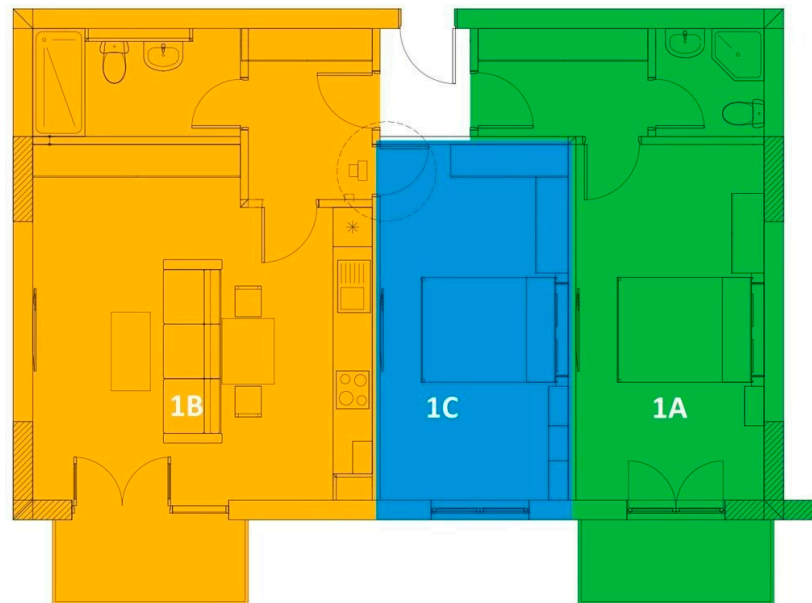
Figure 5. Responsible apartments for generations: two or more completely independent units with the help of enclosing walls [7].
