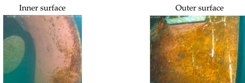
**Figure 10.** Images of biofouling development on the propeller.
