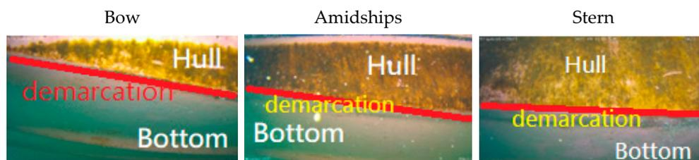
Figure 9. Images of biogrowth demarcation on the ship’s hull and bottom.
