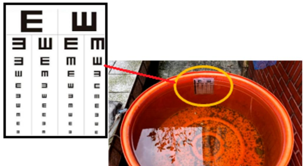
**Figure 3.** Experimental system for establishing the relationship between illuminance and water depth.
