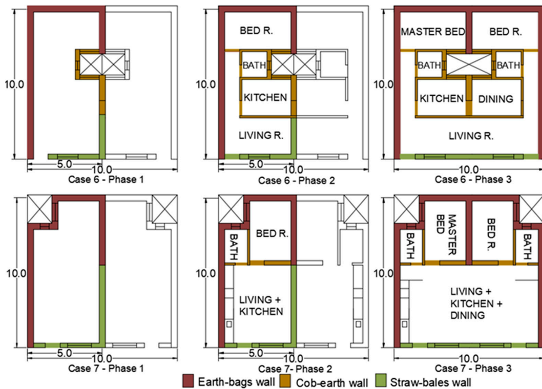
Figure 6. Compact Vertical sited plot layout design Cases (Cases 6 and 7) with their three phases.
