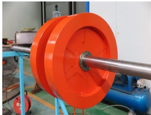
Figure 15. Photo of the generator after sealing.
