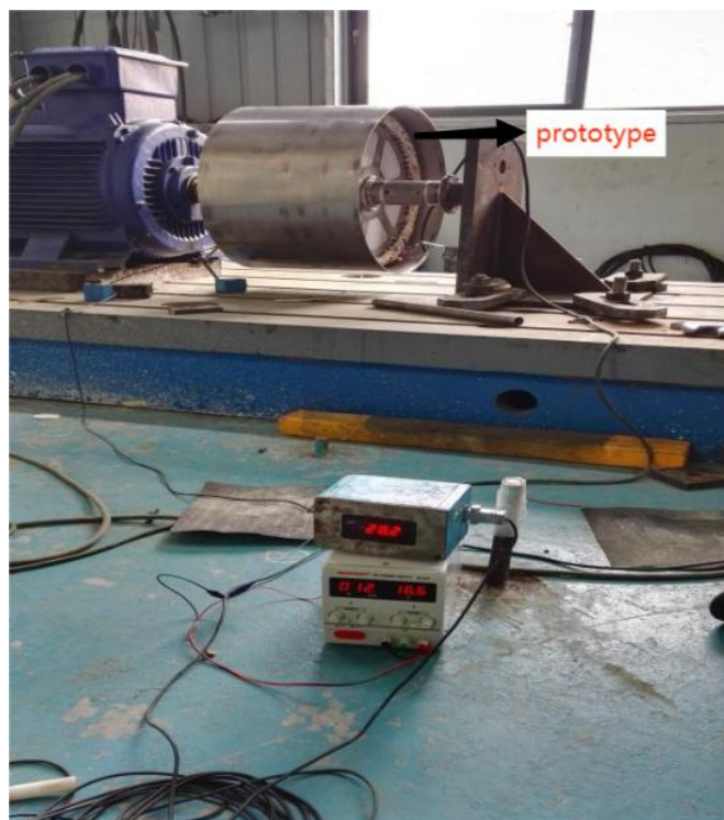
Figure 13. Photo of the motor dragging experiment.
