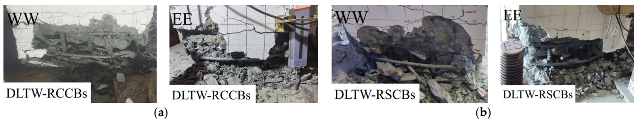
Figure 15. Observed damage of the column bottom for the DLTW-RCCBs and DLTW-RSCBs (drift ratio 4.9%). (a) Specimen DLTW-RCCBs. (b) Specimen DLTW-RSCBs.
