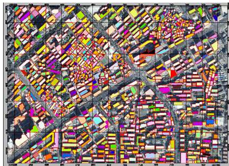
Figure 4. Scheme for image matrix design with grid size \Delta x = \Delta y = 100 m and total row and column numbers of 10 and 13, respectively.
