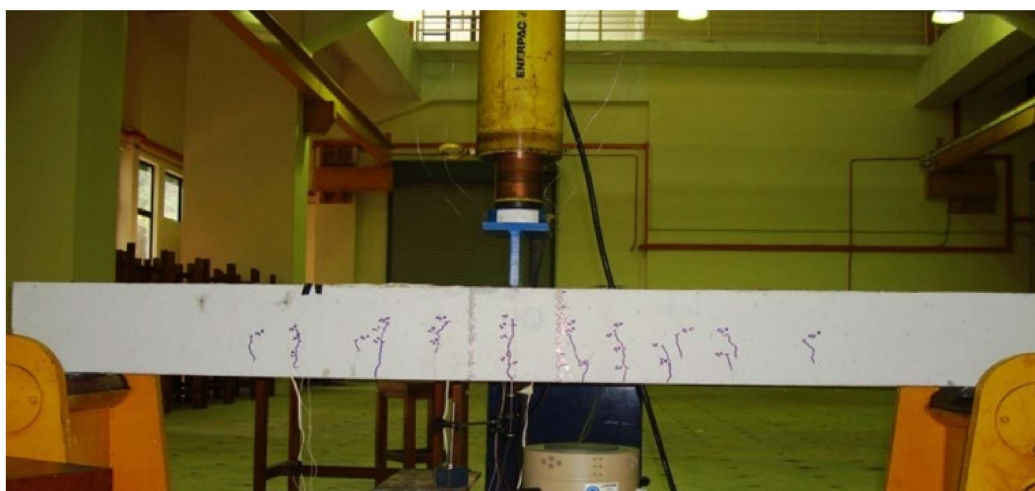
Figure 2. Beam under static test.
