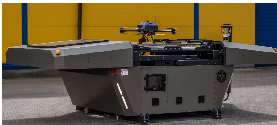
Figure 2. Charging station for automatic docking.
