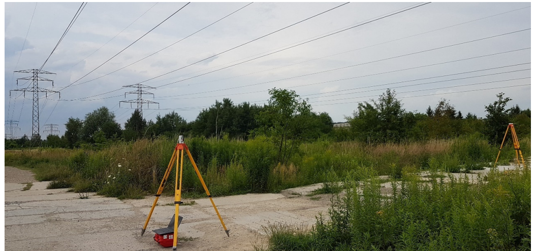
Figure 15. Range test of the MESH network modules under high-voltage overhead power lines.
