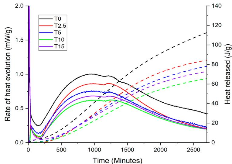
**Figure 5.** Calorimetry of pastes with different TW replacements.
