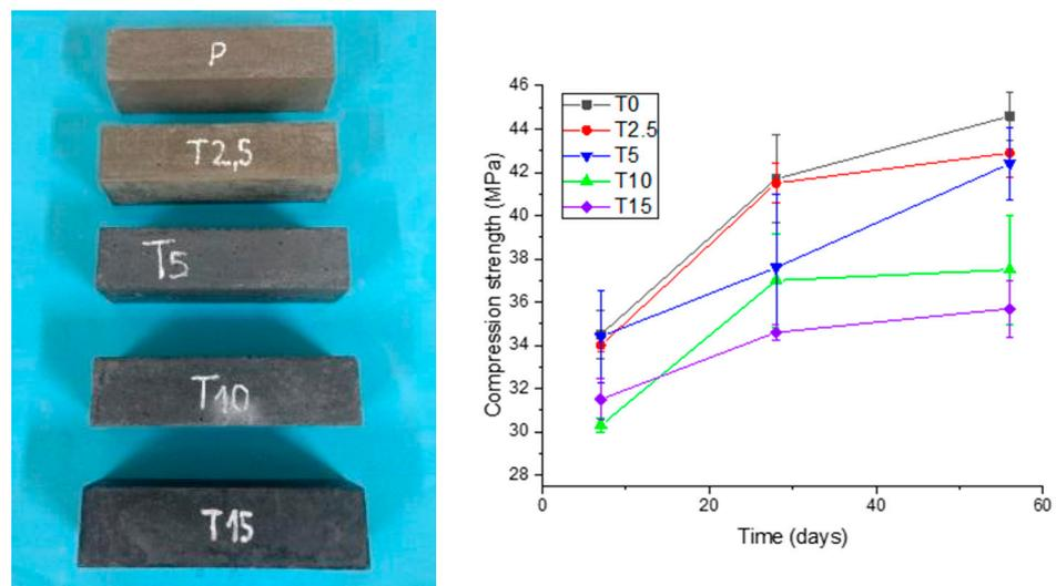
**Figure 6.** Mortars with different TW replacements (left) and compressive strength values (right).
