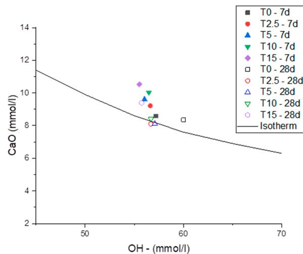
**Figure 3.** Frattini test of pastes with different TW replacements.
