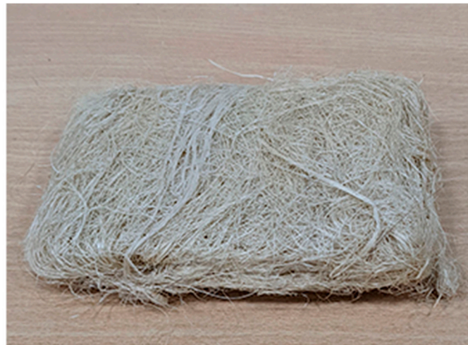
Figure 3. Sample of cabuya fibers that have been prepared according to the specified standards.
