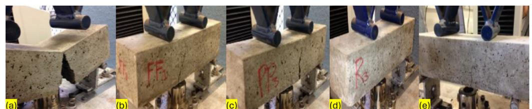
**Figure 17.** Failure behaviour in flexural tests: (a) control (10%), (b) FF, (c) PP, (d) GF, and (e) steel samples.
