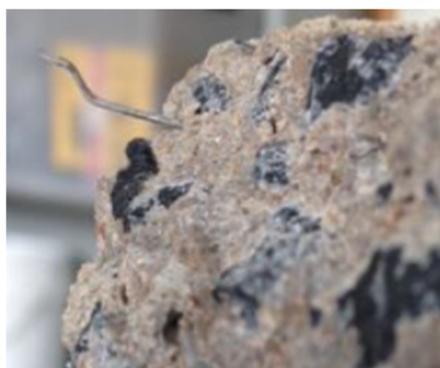
**Figure 33.** Pull-out failure (steel fibre).
