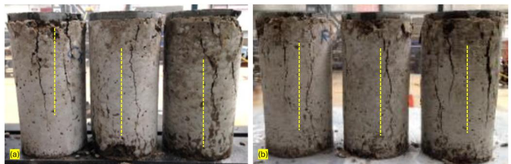
**Figure 14.** Comparison of failure modes of control samples (a) and ReoShore 45 samples (b).
