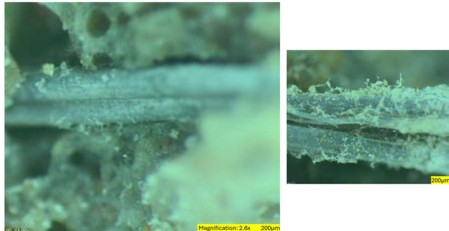
**Figure 20.** Microscopic images revealing the interaction between Forta Ferro PP fibres and the matrix.
