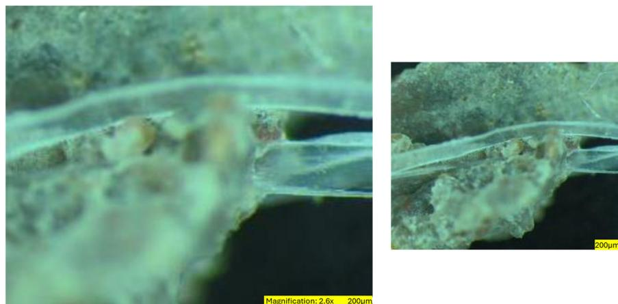
**Figure 21.** Glass fibre–matrix interaction (microscope images).
