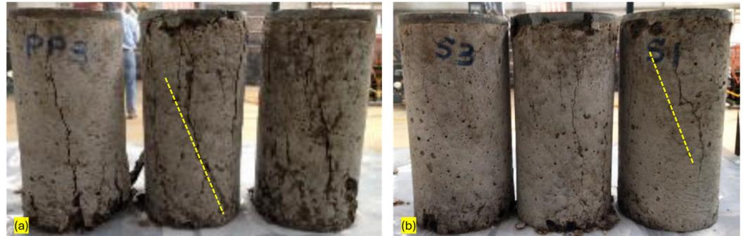
**Figure 15.** Splitting failure of Forta Ferro PP fibre-reinforced samples (a) and steel fibre-reinforced samples (b).
