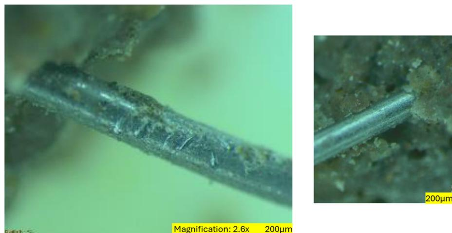
**Figure 23.** Microscopic images showing the interaction of steel with the matrix.
