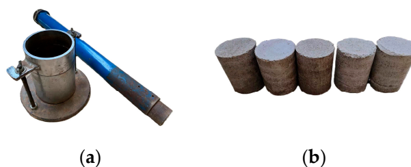
Figure 2. Compaction test equipment and specimens: (a) Heavy-duty compactor and (b) compacted specimens.
