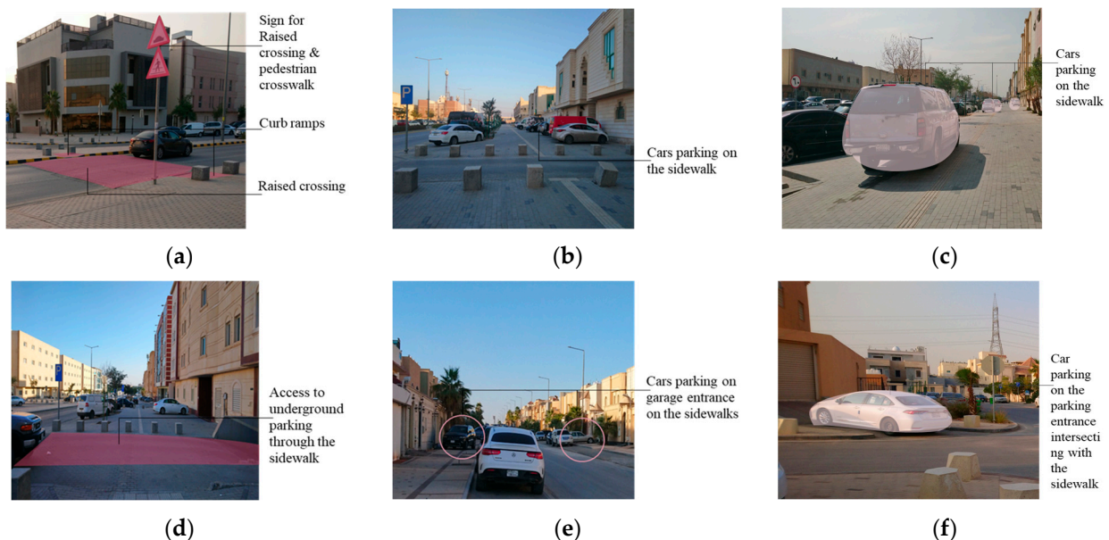
Figure 8. (a) Clearly identified and extensive pedestrian crossings; (b,c) Cars using the sidewalks for parking; (d) Intersecting routes of vehicles and pedestrians interrupting the pedestrian movement; (e,f) Private houses use the sidewalks for parking. Source: Authors.
